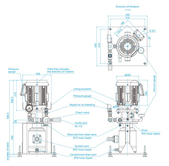
In addition to the parts shown in the figure above, inlet hose, contaminant drain hose, return hose from relief valve, return hose from unloading valve, seal drain tube (3 m each) and hose clamps are included.
