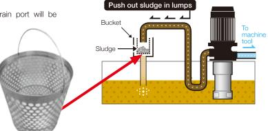
[Simple Layout to Collect Sludge]
